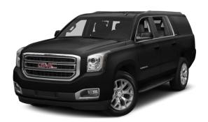
The 2015 GMC Yukon XL is available in three trim levels: SLE, SLT, and Denali. Powering the SLE and SLT versions of the 2015 GMC Yukon XL, a 5.3-liter EcoTec3 V8 engine generates 355 horsepower. The high-end 2015 GMC Yukon XL Denali is propelled by a larger 420-horsepower EcoTec3 6.2-liter engine. The Yukon XL and Yukon receive fuel efficiency ratings nearly identical to the Suburban and Tahoe.
