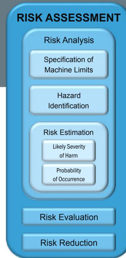
In order to analyze risk, three elements must be combined and considered; the specification of the limits of the machine, identification of hazards, and risk estimation. Together, these attributes are considered to define a level of risk, which is then evaluated to determine whether the risk reduction objectives have been achieved, also known as achieving tolerable (or acceptable) risk.
