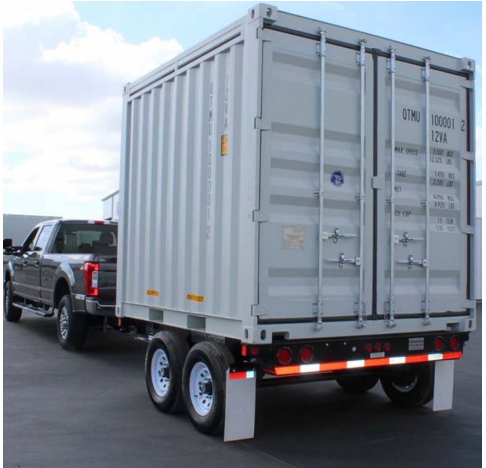
Quantum’s 10-foot modular container has a gaseous capacity of approximately 83,635 Standard Cubic Feet (SCF). Equipped with 6 (or 8) Type 4 CNG tanks, it can be towed by a ¾-ton pickup truck and weighs less than 9,000 pounds empty or 12,500 pounds fully loaded.
