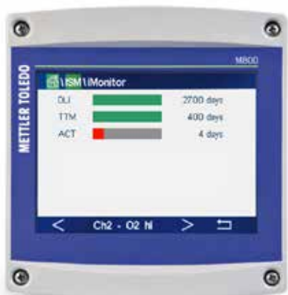
Figure 1 - iMonitor screen showing predictive diagnostics for a pH electrode
