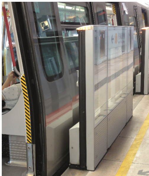
Figure 16 – Example safety edge applied for clamping/crushing contact hazards
