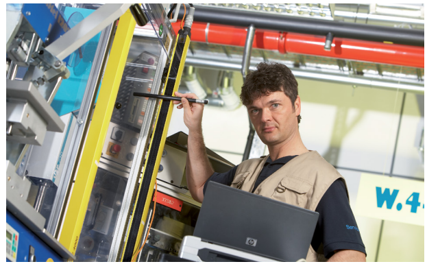
Figure 7 – Testing effective detection capability of a safety light curtain
