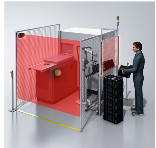
Figure 6 – Example of vertical presence sensing devices (area scanner and light curtain)
