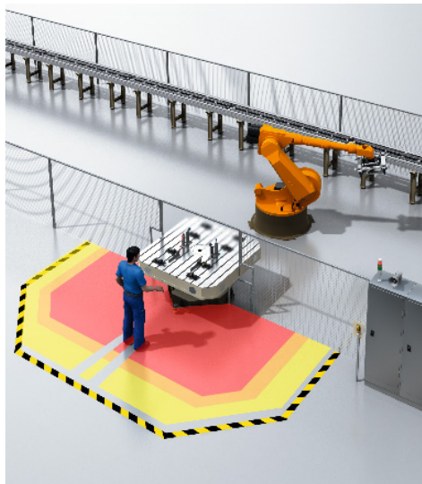
Figure 9 – Example of a horizontal presence-sensing device (area scanner)
