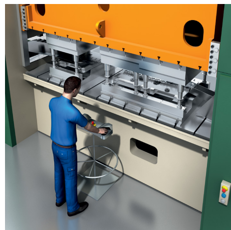
Figure 11 – Example of a two-hand control device
